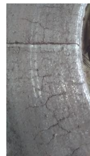
Figure 10. Cracks caused by thermal overload
