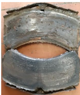
Figure 8. Abrasive and thermal overload (truck without retarder)
