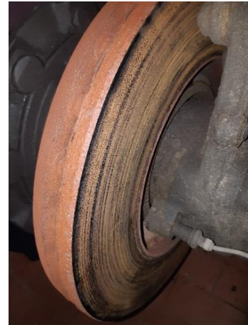
Figure 3. Wear on the brake disc and brake pads
