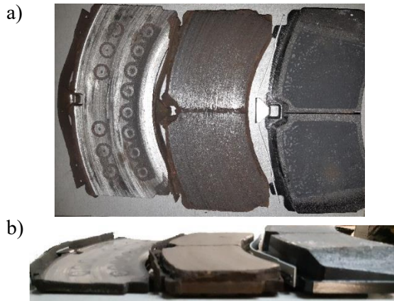
Figure 2. Excessive wear of the interior brake pad a)Top view; b)Side view
