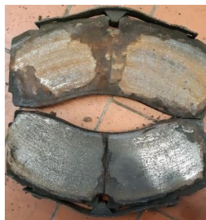
Figure 9. Corrosive wear 132,000 km / 2 years
